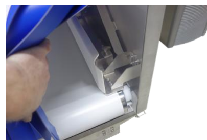
Interior View of Conveyor Belt
