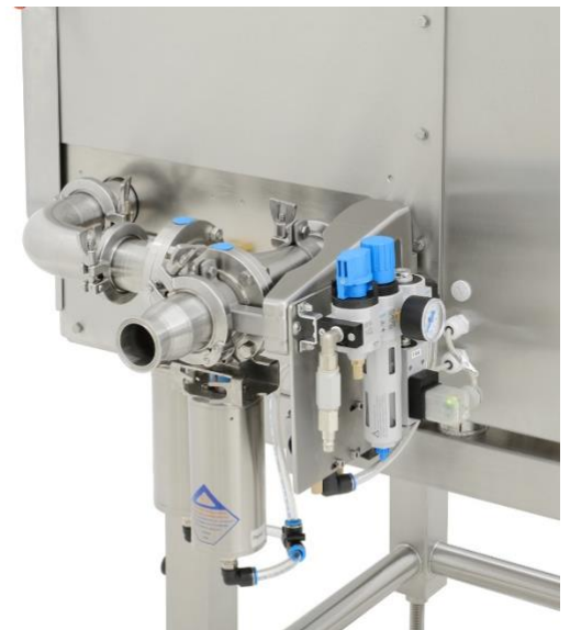
XRAY SHARK® XD08-H1-PIPE with air pressure reject system.
